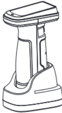
Put the instrument into the calibration base for white calibration.
