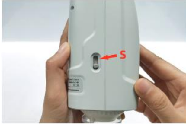
Small aperture switch to "S" display
